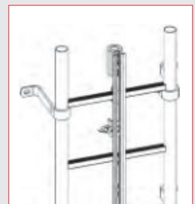
When using the counter bracket an additional movable bottom end stop (order no. 0529 4007 00) has to be assembled (not included).
