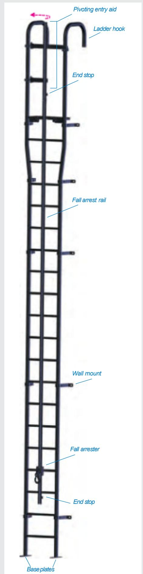
By contrast with ladders with safety cage, ladders with fall arrest equipment are not subject to any height restrictions and provide real protection against fall from heights.
