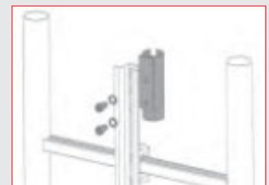
When using the counter bracket an additional movable bottom end stop (order no. 0529 4007 00) has to be assembled (not included).
