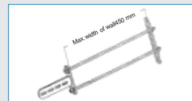
1 set of anchor bolts is required for 1 wall connection element
