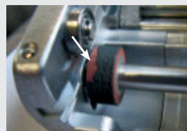
b V-Marking for wear and tear on the friction wheel
