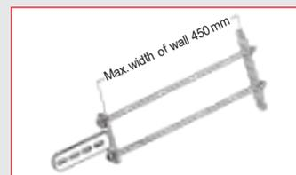
1 set of anchor bolts is required for 1 wall connection element
