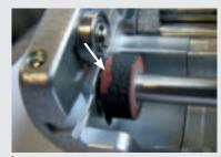
b VMarkingfor wear and tear on the friction wheel red = exchange necessary
