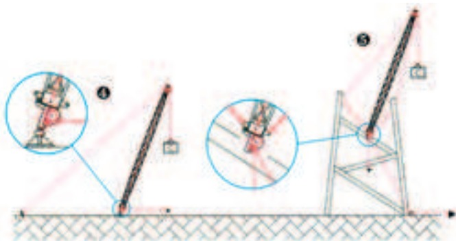
EXAMPLE OF A PROPER USE OF AN INTERNAL ROPE-PASSAGE GIN POLE
