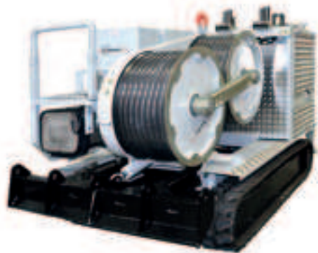
Self-propelled puller-tensioner 70 kN
