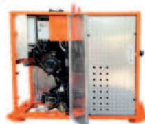
Dismantlable puller-tensioner 70 kN
